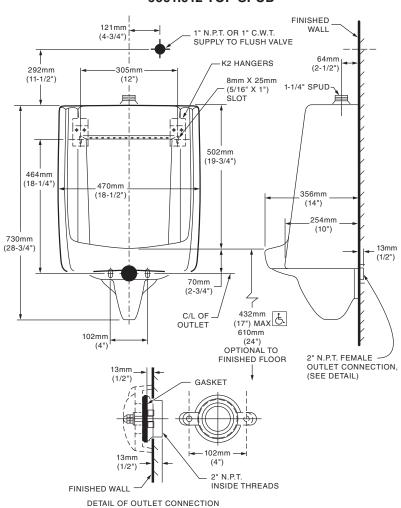
**NOTES:** FLUSH VALVE NOT INCLUDED WITH FIXTURE AND MUST BE ORDERED SEPARATELY. PROVIDE SUITABLE REINFORCEMENT FOR ALL WALL SUPPORTS.
